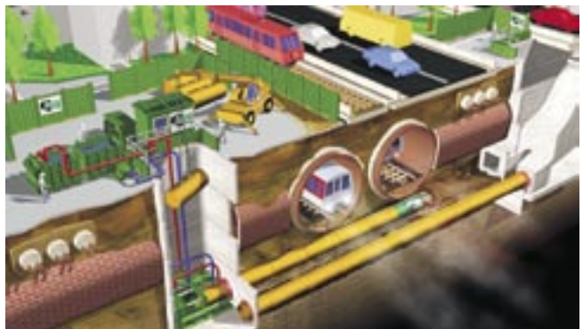
Fig. 8. Microtunnelling method applied to reconstruction of the duct colliding with the tunnels under construction
